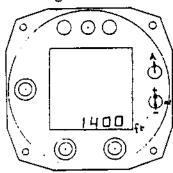
STEP 2 Enter Distance-to-Go using IN Switch
